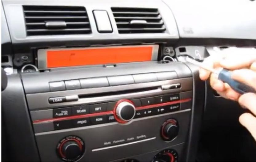
Step 3: Lift the front edge of the top panel with the air-conditioning vents to pull the radio out.
